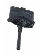
FIST Gel Sealing Kit for oval splice closure port, sealing 1 looped cable with diameter between 16 and 20 mm
