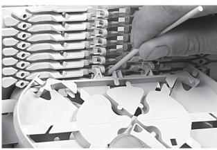
4.4 To remove the tray put the fiber guiding pin between lip onwraparound groove plate and tray and move lateral towards \$1.
