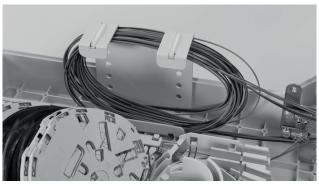
2.2 Store the looped tubes into the loop bracket.
