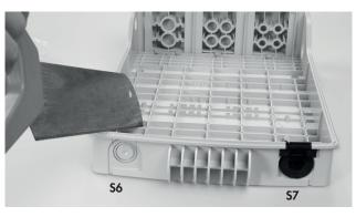
1.3 Use a hacksaw to reach the onion rings, which can be opened with a plier to open the in-line ports (S4/S5).
