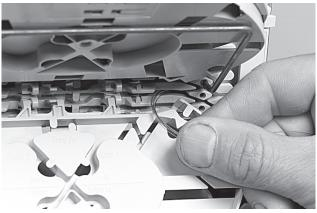
4.5 Position the wedge carefully such that the groove is stillaccessible for the fibers and be careful not to push the wedge againstfibers. To remove the wedge, use two hands to pull on both ends (nearthe groove plate). Route the fiber in the grooves of the wraparoundgroove plates to the entrance of the identified tray. Fiber must berouted in the groove below the hinge of the tray!
