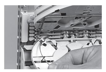
4.6 Pull gently on the fibers in the tray and make sure that the fibersare well contained in the routing block and wraparound groove plate.
