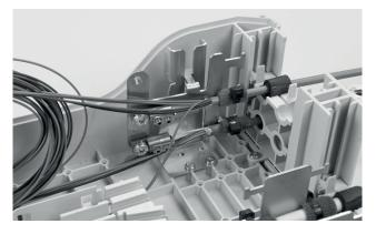
2.1 Install the looped cable into the ports.
