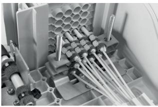
3.1 Install the drop cables into the ports.
