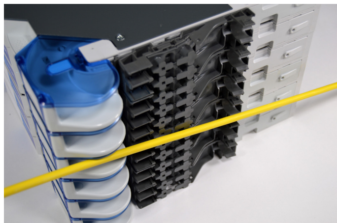
5.5.1. A high fiber count loose tube cable can be routed with a maximum of 6 FACT elements. Use the CTU bracket mounted in the middle of the row for mounting the cable. Route and divide the loose tubes via the shortest and most bendless way to the different CTU elements.
