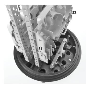
**16 PORT BASE**: Ports (1+3+5+11+13), (2+4+6+12+14) for cables to (S2). Ports (5+7+9+15+17), (6+8+10+16+18) for cables to (S1). Verify the position of two cables if they are placed on the same side (next to each other) because the total amount of loose tubes in ports going to one tubeholder can never be more than mentioned in the capacity of the tubeholder.
