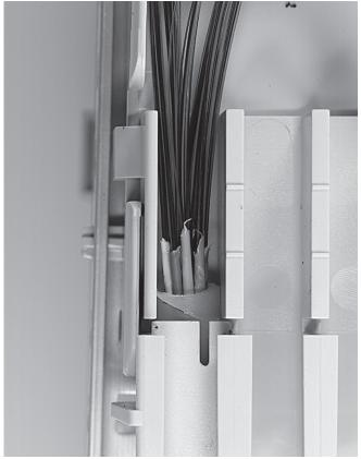
4.2.27 Match the spiral tube on the tubeholder, mark and cut the spiral tube from this mark. Remove element per element the ID cords or compact cable sheet (Microgain<sup>™</sup>, Compacttube<sup>™</sup>, ...) till about 10 mm after the spiral tubes; use PTFE tape to bundle the fibers and the ID cord. Position the small spiral tubes in the respective tubeholders. Bottom picture shows compact cable sheet.
