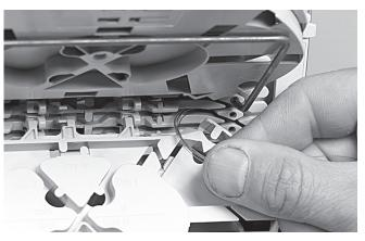
6.7 Route the fiber in the grooves of the wraparound groove plates to the entrance of the appropriate tray. Fiber must be routed in the groove below the hinge of the tray!
