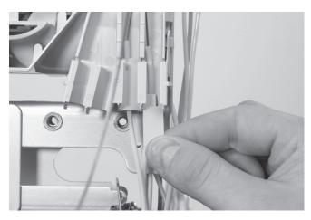
4.1.18 In case of **Reversed oscillating cable** Identify exchange and customer-side using some PTFE tape around the fibers. One can also use the FIST-split-collets-rings markers to identify the loose tubes.
