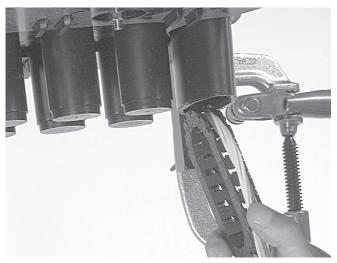
4.1.11 Push the loose tubes (looped around the LCIT) through the oval port. Remove the LCIT and pull the cable gently in the closure.
