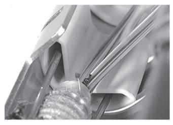
4.2.7 Insert the strength members from the cable into the strength member stop. Secure the cable with the hose clamp onto the loopbracket. Secure the cable with tie wrap onto the loopbracket Secure the screw of the strength member stop on the loopbracket. Wrap a few layers of tape around the hose clamp.
