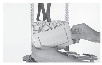
6.1 Remove the hook and loop fastener and routing block cap. To remove the routing block cap lift the two snaps at one side of the routing block cap.
