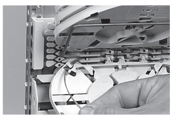
6.8 Pull gently on the fibers in the tray and make sure that the fibers are well contained in the routing block and wraparound groove plate.
