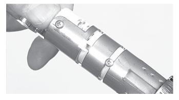
4.2.25 Slide the loop breakout device in the loopbracket and secure the two screws. Open the oval port as described in loose tube preparation.Take the oval sleeve and place the packing bag that has been opened on both sides in the oval sleeve to protect the hotmelt inside the sleeve against dirt and grease. as discribed in loose tube preparation.
