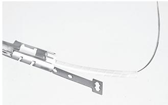
4.2.35 Insert the spiral tube over the fibers into the breakout till the tube stop.
