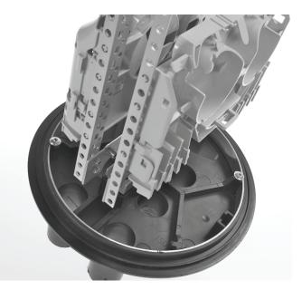
**6 PORT BASE:** Ports (1+3), (6+8) for cables to (S2). Ports (5+7), (2+4) for cables to (S1). Verify the position of two cables if they are placed on the same side (next to each other) because the total amount of loose tubes in ports (1+3) or (2+4) or (5+7) or (6+8) can never be more than mentioned in the capacity of the tube holder.
