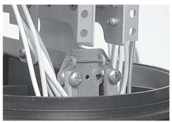
4.1.12 Position the loop bracket in the bottom bracket and lock with the split pin.
