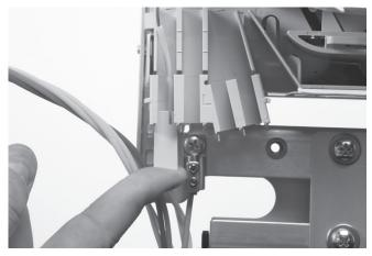
4.1.31 Position one or more loose tubes in the tubeholder according to the correct position and slide the tube holder retainer with the snap forward in the lowest possible cavity of the tubeholder above the loose tube. The tube holder retainer must snap. (see capacity of tubeholders).
