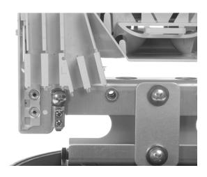
4.1.23 Secure the strength member connector in the closure (on the bottom bracket )
