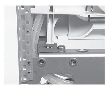
4.2.22 Place cover back in place, Make sure the cover is under the lip of the bottom island. Hinge the basket inbetween the UMS profiles and make sure the hinge is in the correct position.
