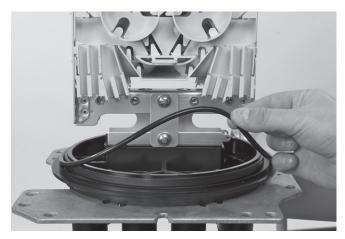
3.2.1 Open and remove the clamp. Remove the dome and the O-ring Remark: be carefull with the O-ring and the sealing surfaces on the base and dome (avoid damaging). Clean only with clear water or with the cleaning tissue, included in the kit, if needed
