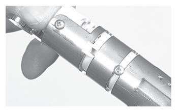
4.2.6 Slightly loosen the screws of the two strength member stops on the loopbracket such that one can position the strength members stops according to the position of the strength members.
