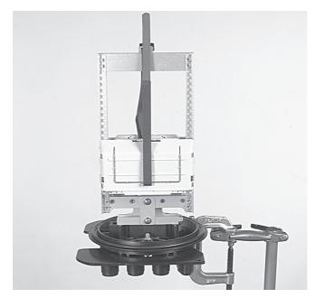
3.1.1 The FIST-GCO2 will be mounted temporary on the work-stand. The work-stand is wrap-around, so that the FIST-GCO2 installed with cables can be taken away from it.
