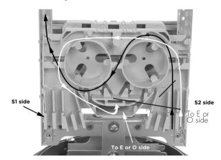
Fibers can be routed between OS1, OS2, ES1 and ES2. In case that fibers have to be routed from SIDE-O (Odd portnumbers) to SIDE-E (Even portnumbers), use the window (see picture). Select the cable termination as such, that a minimum of fibers will cross and have to be routed through the window. Therefore the selection of the ports according to the cable lay-out is important.
