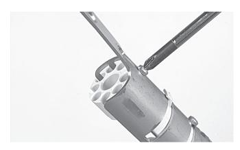
4.2.32 Loosen a little bit the screws such that one can position the strength members stop according to the position of the strength members and remove the break-out part.
