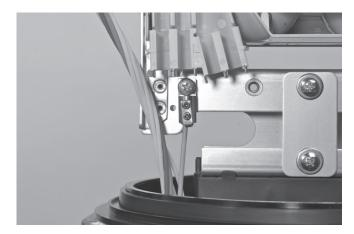
4.1.25 Push the loose tubes in the port and secure the strength member in the strength member connector. Be sure that all loose tubes are routed without crossing around the strength member.
