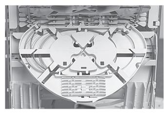
6.9 Store the fibers temporarily on a tray (picture shows the case of a loopback).
