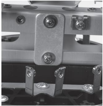
4.2.40 Secure the strength member plates in the closure. Use FACC-DSCT for dual strength member cables.
