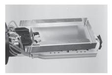
16.1 Slide the FOSC-A-BASKET onto the tray support and secure with screw. Coil the ribbon fiber or bear fiber (e.g. central core cable) with the basket and secure.
