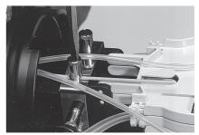
**11.5** Install the screw and the washer into the strength member fixation device. Slide the cable strength member under the washer and tighten the screw. Cut away the excess length of the strength member.
