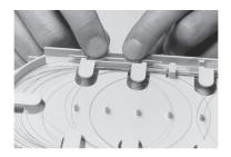
7.1.6 For 8 fiber capacity tray, two fusion protection sleeves should be installed on top of one another in one splice holder.
