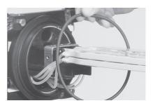
**9.3**. Ensure seal areas and sealing ring are clean and sealing ring is in place at the base.
