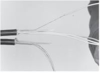
**5.1** Remove the cable sheath (and shield if present) over a length as required by locally approved practice (e.g. 1,2 meters). 1.1 m is the maximum allowed length if the ribbon (4R4) or high capacity trays (S16) are used. Clean filling compound from fiber tubes and cut central strength member at a distance of 75 mm from outer jacket.
