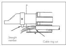
**5.4** Align cable ring cuts with edge of base.
