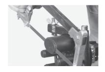
**4.2** Install the FOSC in the FOSC-STAND and open the oval port for cable entry by cutting the port at the ridge with a hacksaw. Deburr the inner edge of the port opening with abrasive strip.
