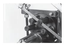
**11.1** Open the port for cable entry by cutting the port at the ridge with a hacksaw. Deburr the inner edge of the port opening with abrasive strip.
