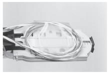
**15.2** Insert the unused buffer tubes into the loose tube storage sleeve. Use tie wraps to secure the storage sleeve.
