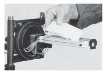
**9.2** Open and remove the desiccant bag from its package and place the desiccant bag on the upper tray. Secure the desiccant bag onto the trays with tape.
