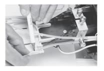
7.1.1 Each splice tray accommodates 8 fiber splices maximum and each side of the tray holds a maximum of 4 big transportation tubes.
