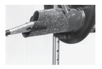
**6.6** Shrink the oval cable seal on the FOSC-base side with the recommended hot air gun device with reflector. Shrink sleeve until the green thermo-indicating paint is converted to black. (Make sure the hot-air temperature is at least 350°C).
