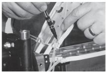
**8.2** Proceed for fiber splicing as described from point 7. However, provide enough slack on transportation tube such that no severe bending or kinking of tube may occur during hinging.
