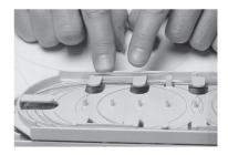
7.1.5 After each splice is made, the splice should be stored in the splice holder. Do not deform the splice protector during insertion. The fiber slack should be coiled into the tray.
