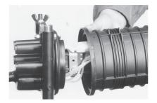
**10.2** Remove carefully the dome avoiding damaging the sealing ring and fiber management.
