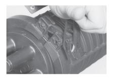
**9.4** Place the dome carefully over the trays onto the base. Put the clamp around the base/dome interface. Close the clamp.
