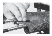
**6.5** Slide the oval cable seal over the oval port. Install the branch-off clip. Check that the heat-shrinkable sleeve butts up against the FOSC-base and the branch-off clip is completely inserted. Tape the two cables together.
