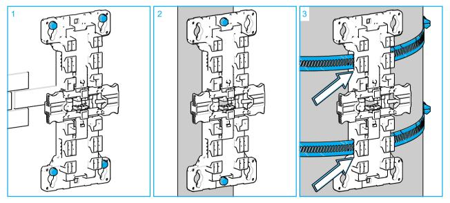
Mount the UMB on a flat surface with 4 screws.
